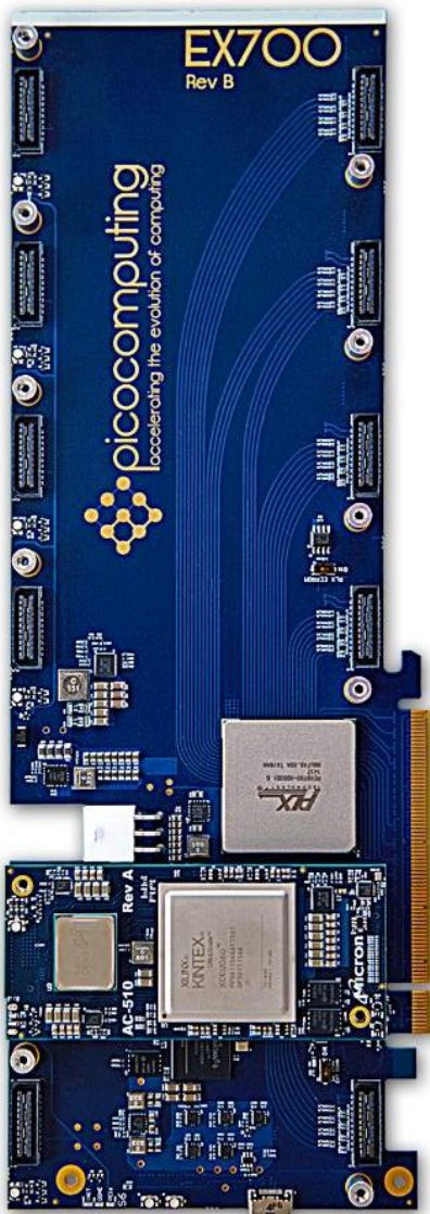
EX-700 Backplane shown with a single AC-510 module (purchased separately) attached for illustration purposes.
